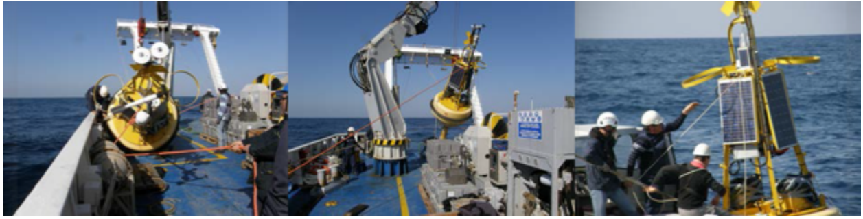
Figure 3.1 a: Oceanographic buoy recovery on the ship's stern during mooring maintenance procedures.
