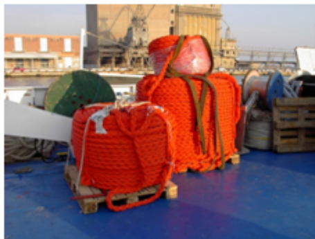
Figure 1.2.2 c: Synthetic mooring line
