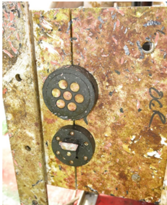
Figure 2.3 a: Irradiance sensor after a one-year deployment during which the bioshutter broke.
