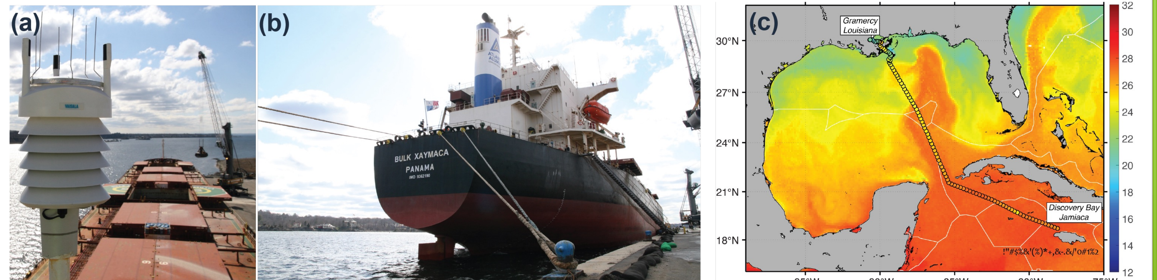
Fig. 4: a) Xaymaca's Vaisala WXT-536 transmitting NRT data; b) M/V Xaymaca; c) CMEMS sea surface temperature (4-day average: April 20-24, 2022) with Xaymaca's NRT in situ air temperature along the ship track superimposed. In January of 2021, a Vaisala weather station (Fig. 4a) and 75 KHz ADCP were installed on the Pangaea Logistical Systems Ltd. vessel M/V Bulk Xaymaca (Fig 4b) running a roundtrip between Jamaica and New Orleans about every 3 weeks (Fig 4c).
