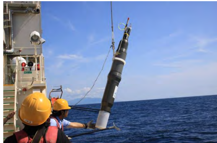
Deep Ninja float (4000m) with turbulence sensor Tsurumi/RSI/AORI
