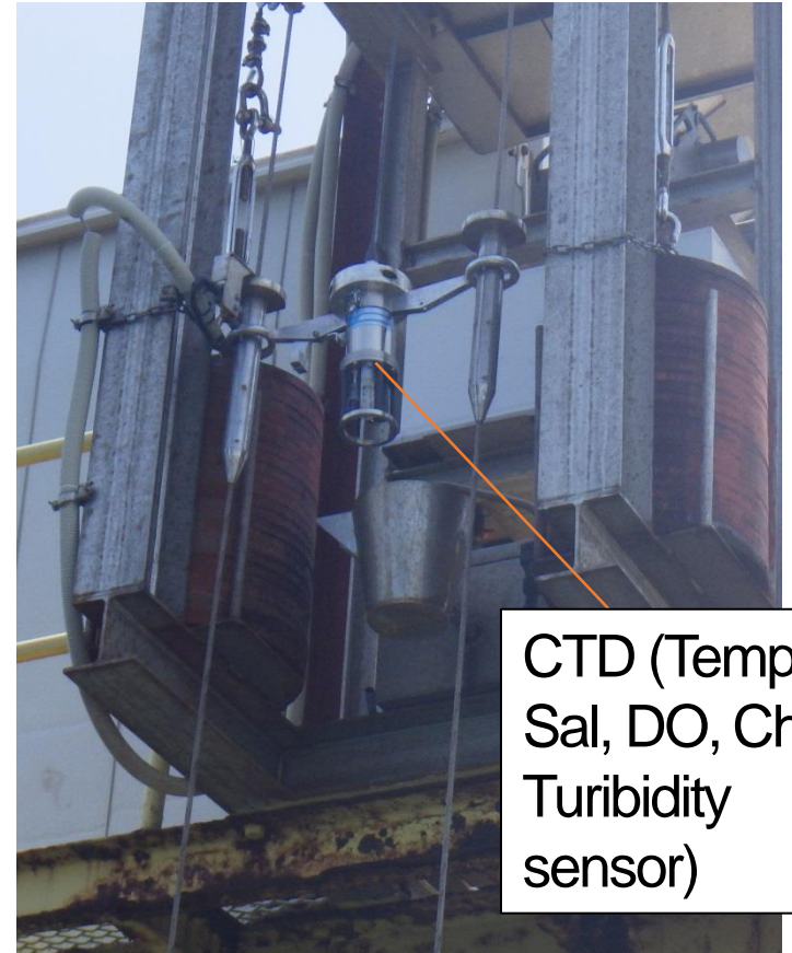
Automatic vertical profiling system of water quality
