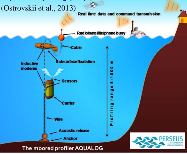
Multisensor platform for autonomous vertical profiling in the ocean (P.P. Shirshov Institute of Oceanology, RAS).
