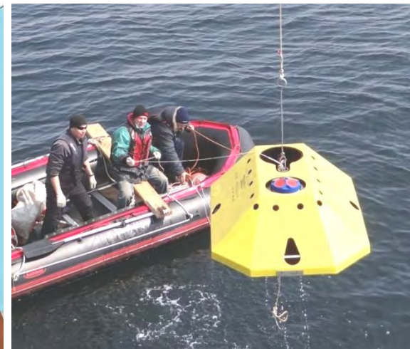
Moorings with T, S, DO, Turb, Flu and current meters (SBE37, RBR-XR, S4, Infinity EM, RDCP600, WHS300)
