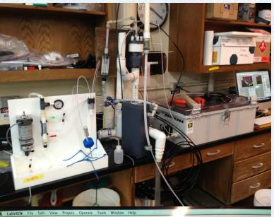
Combined pCO<sub>2</sub>/TCO<sub>2</sub> measurement on continuous flow and/or discrete samples (aka 'Burke-o-Lator').
