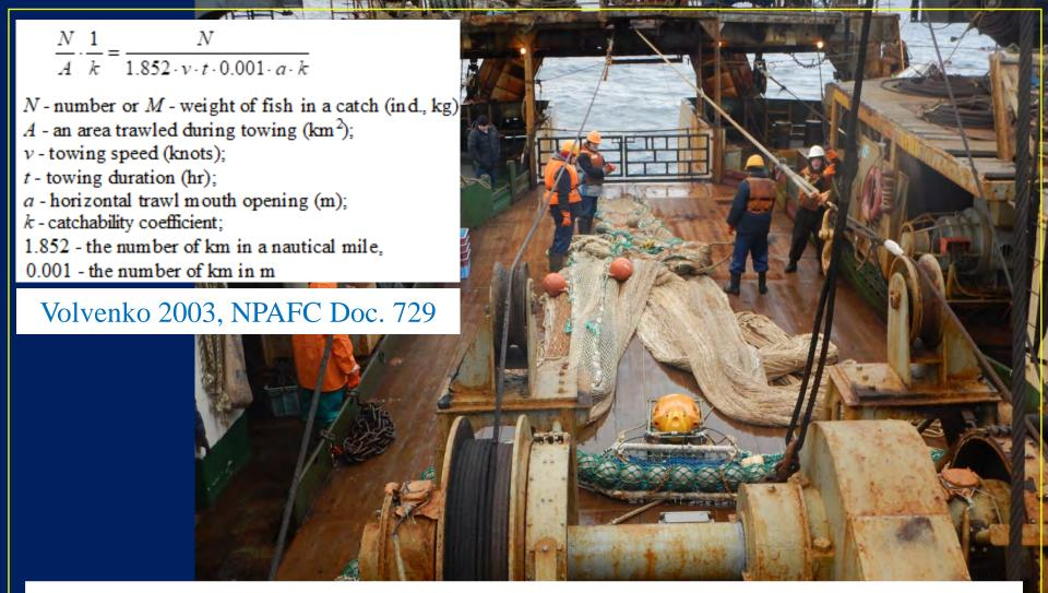
Used gear: surface (0–30 m) midwater trawl 80/396 m (opening ~120 m<sup>2</sup>, 30m depth x 40m width) for one hour at a speed of average **4.5** knots
