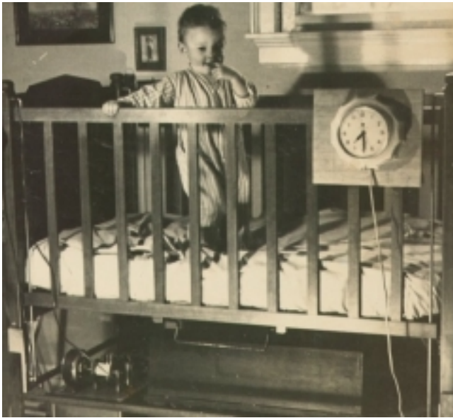
Fig. 2 Mike in 1939, at age of 16 months, with comograph attached to his crib mattress to monitor his sleep.
