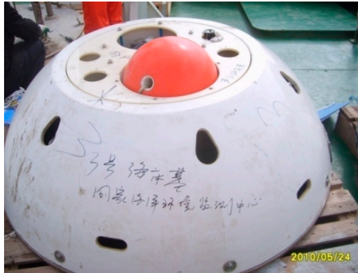
Figure 2: The seabed platform observation system
