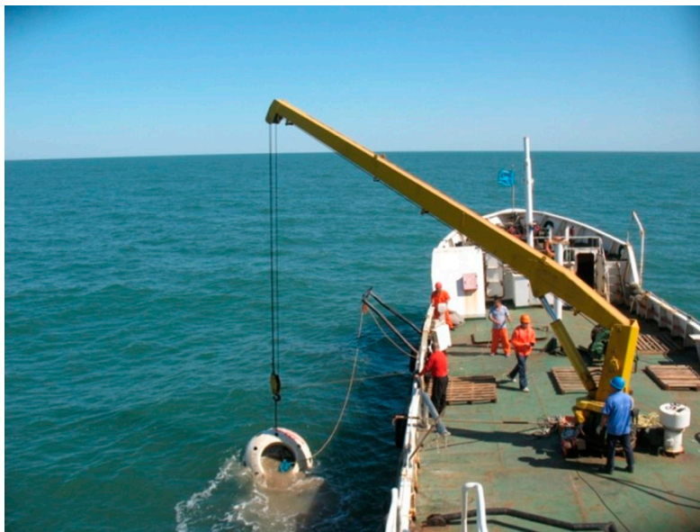
Figure 3: Retrieval of the seabed platform observation system
