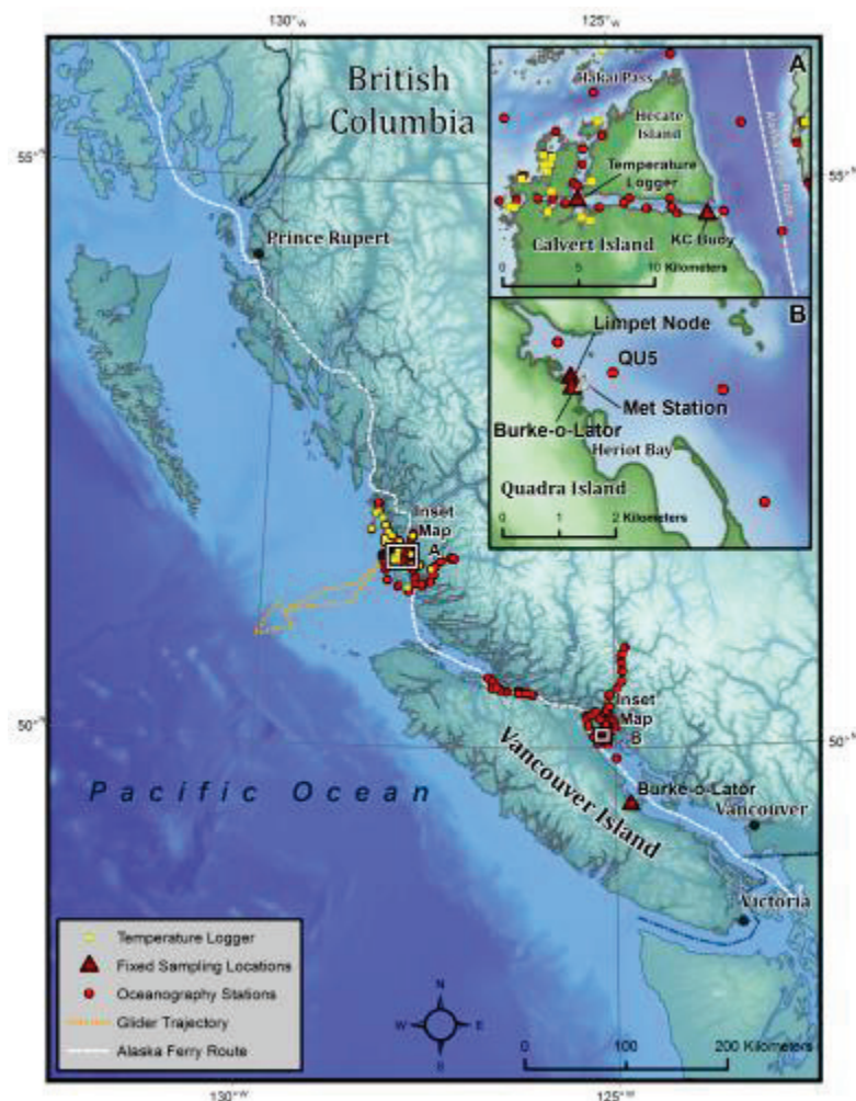
Figure 2. Locations where the Hakai Institute collects ocean data in British Columbia. Hydrographic stations (red circles) are where physical, biological and chemical measurements are made at bi-weekly to monthly frequencies. High frequency data from fixed sampling locations (red triangles) and temperature loggers (yellow circles) are output every 5 minutes. Instrumentation on board the Alaska Marine Highway System (AMHS) M/V Columbia measures surface parameters while underway every 2.5 minutes along weekly ~1000 nm transits between Bellingham, Washington (48.75°N) and Skagway, Alaska (59.64°N).
