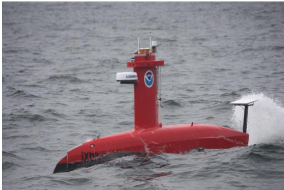
Figure 21. DriX uncrewed surface vehicle underway during tests in Alaska (photo Alex De Robertis).
