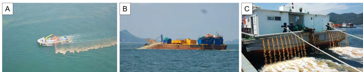
Figure 8. Various methods of clay dispersion for HAB removal in Korea. (A) 2G clay dispenser; (B) 3G clay dispenser; (C) Spraying modified clay
