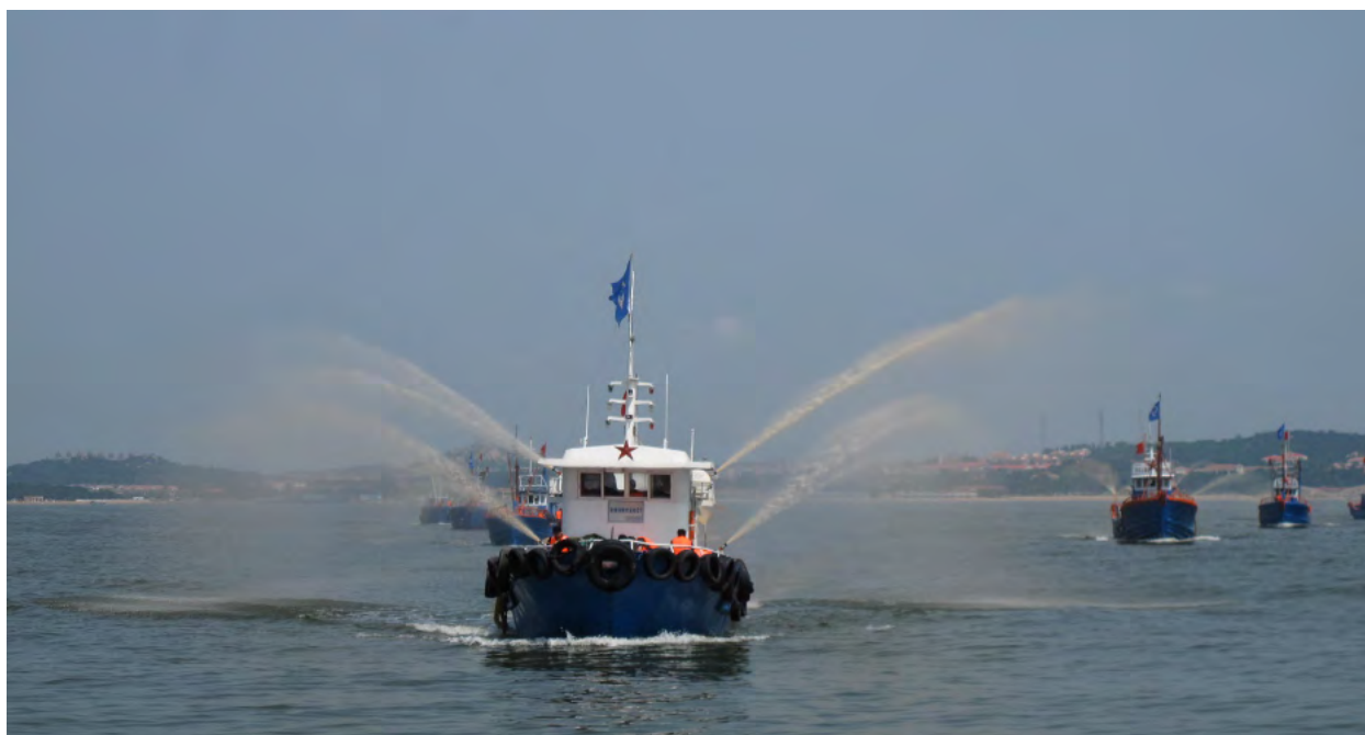
Figure 10. Large scale HAB suppression using MC in open (oceanic) waters in China
