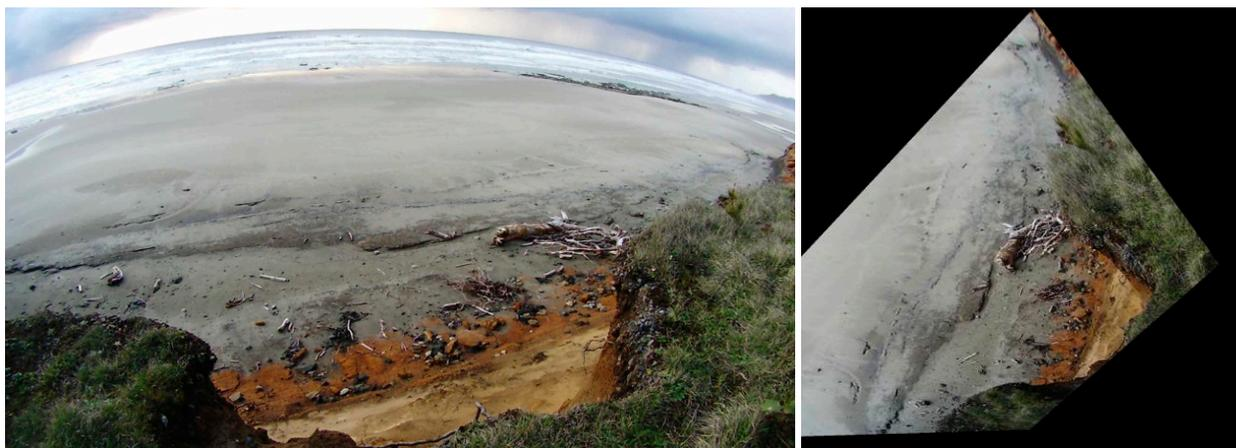
Fig. 10 Original photograph taken by webcam (left panel) and photograph after applying the projection transformation method (right panel). Image provided by Atsuhiko Isobe, Kyushu University.
