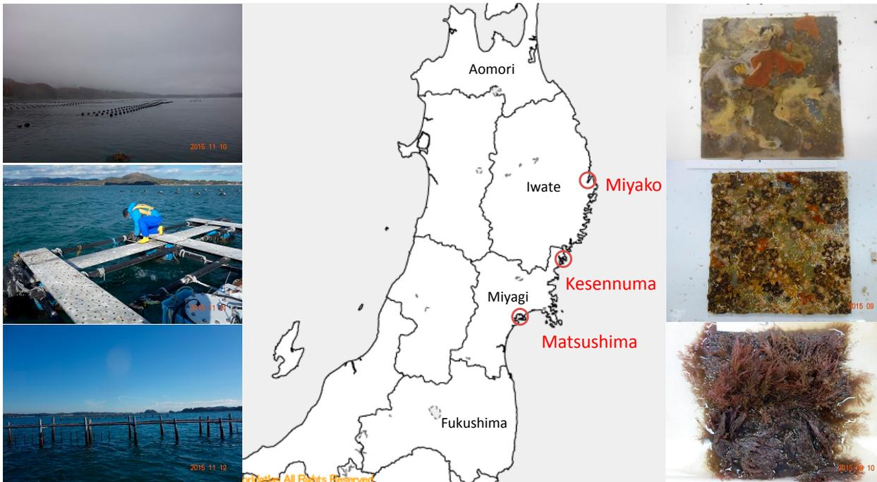
Fig. 12 Map of fouling panel deployment sites in the Tohoku area of Japan (middle), site photographs (left) and examples of the fouling panels from each site after a 1-month deployment (right). Image provided by Karin Baba, Japan NUS Co.
