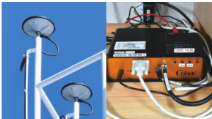
Figure 4: Precipitable Water Vapor measurement system.
