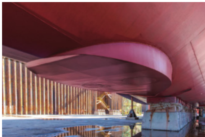
Figure 5: Precision Depth Recorder and Acoustic Doppler Current Profiler (ship's underside).
