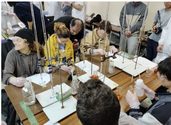
Dissolved oxygen analysis by titration method. Photo credit: Daiki Nomura
