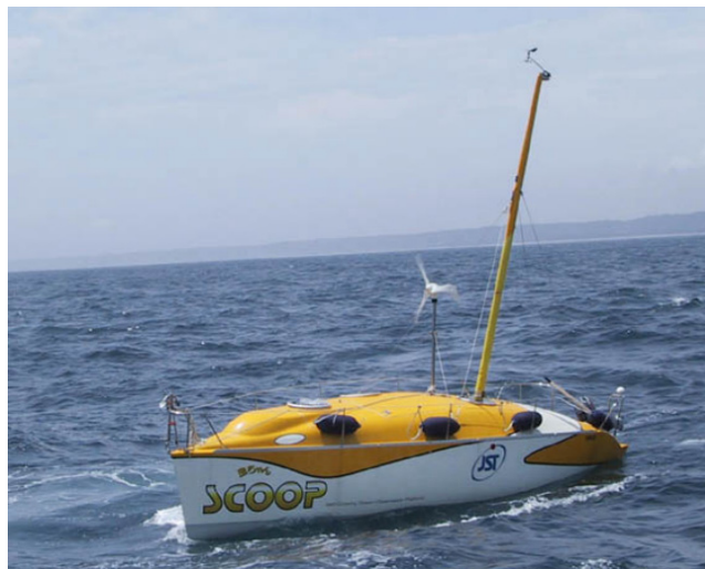
Fig. 3 Self Cruising Ocean Observation Platform (SCOOP) nicknamed “Kan-chan” in Japanese. The boat is made of FRP with a length of 8 m and a maximum width of 2.8 m. It is powered by a diesel engine, which drives DC and AC dynamos. SCOOP is propelled by the DC motor and travels at a speed of 2-4 knots. It contains two 700 l fuel tanks that enable 700 hours of continuous operation without maintenance. We can control SCOOP and obtain real time observing data and CCD pictures via satellite communication systems (N-Star and ORBCOMM). SCOOP is equipped with an atmospheric autonomous measurement system, including the newly developed micro flow injection analyzers for SO 2 and NH 3 , and a dichotomous aerosol filter sampler with an absorption spectrometer for elemental carbon and a beta absorption detector for mass concentration. Simultaneously, vertical profiles of temperature, salinity, chlorophyll fluorescence and turbidity can be obtained by a Yo-Yo system.
