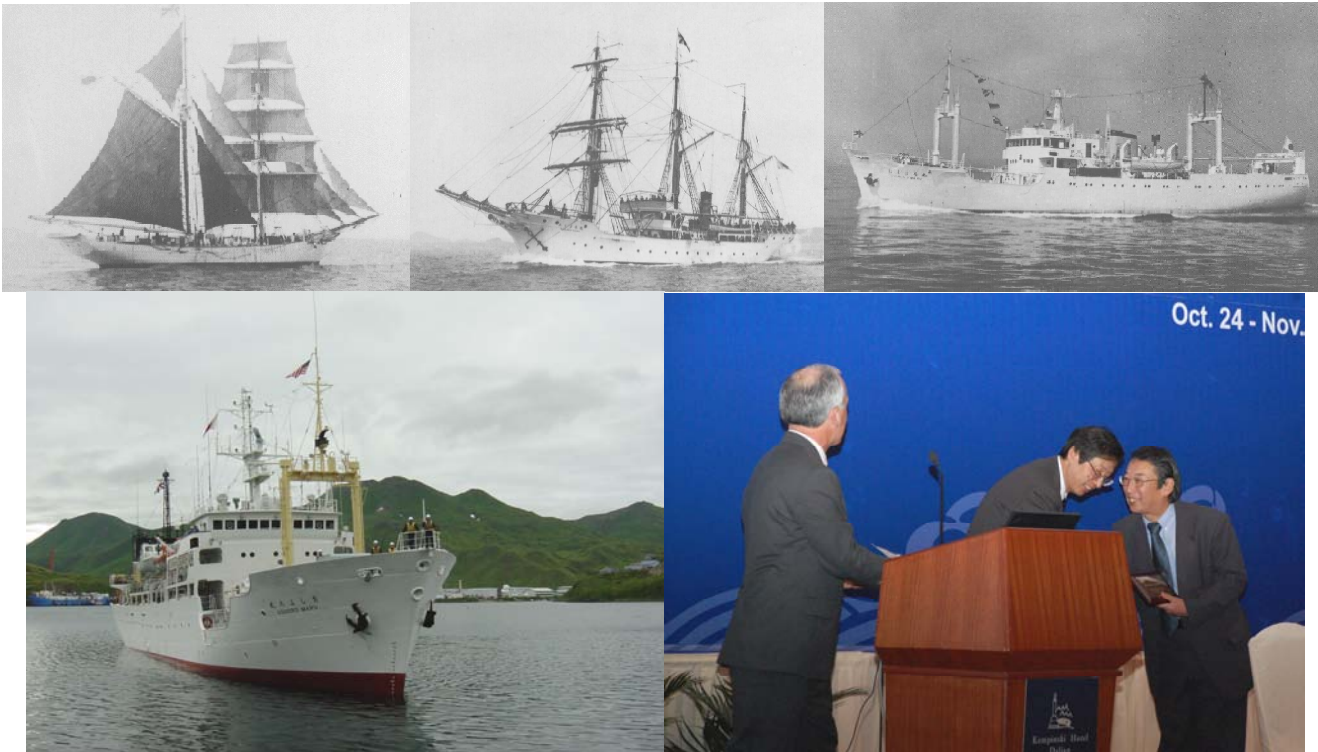
Top row, left to right: the Oshoro-maru I as a 31-m wooden brigantine built in 1909, the Oshoro-maru II as a 42-m steel barkentine built in 1927, and the Oshoro-maru III as a 67-m 1,180-ton stern trawler built in 1962; bottom row: the Oshoro-maru IV as a 73-m 1,383 t stern trawler built in 1984, and the 2008 POMA presentation ceremony (Dr. John Stein on the left, Dr. Tokio Wada in the centre and Dr. Akihiko Hara on the right).
