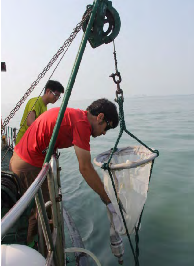
Photo 6 Students collecting water samples from the CTD Niskin bottles (top) and a net deployed to sample phytoplankton and zooplankton (bottom) during the cruise hands-on practicals on board the R/V Ocean II in the Jiulong River Estuary.
