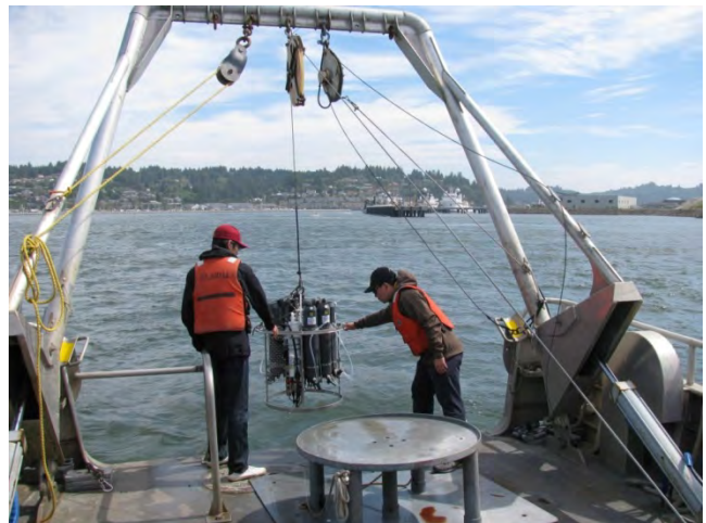
Photo 3 Hiromu Ishiyama (Japan) and Sung Yong Kim (Korea) deploy a CTD rosette from the R/V Elakha . Photo by Jack Barth (OSU).
