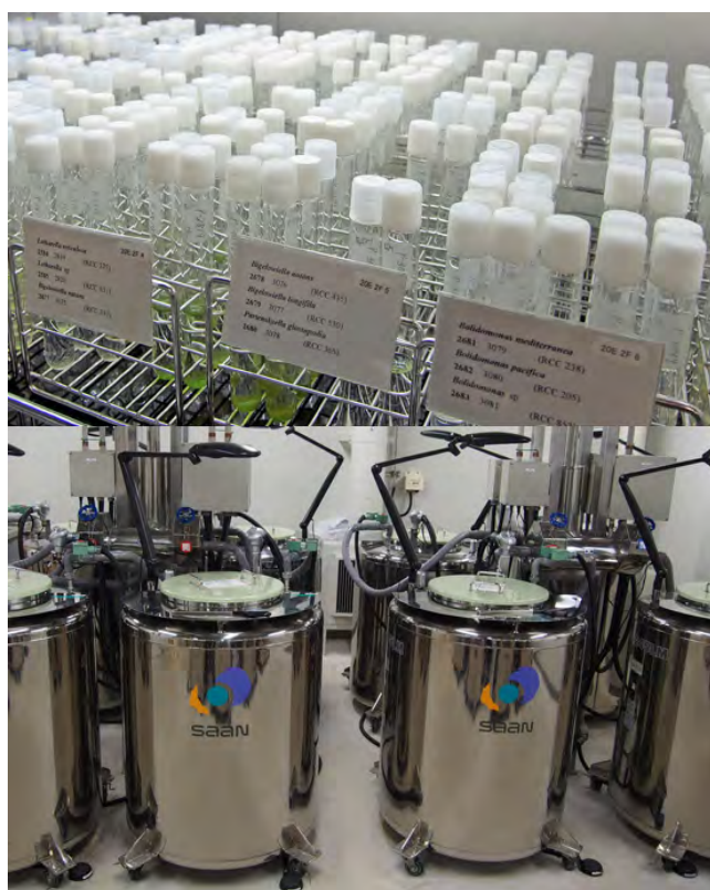
Upper: Subculture of strains in liquid or agar media. Lower: Cryo-preserved strains in liquid nitrogen tanks.
