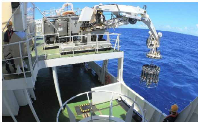
Figure 4. Full-depth oceanographic observation in the summer of 2021 along 24°N in the western North Pacific by JMA.
