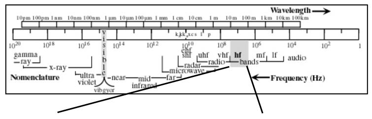
3-30 MHz (between AM radio and TV) Wavelength ( $\lambda_r$ ) : 10  $^{\sim}$  100 (m)
