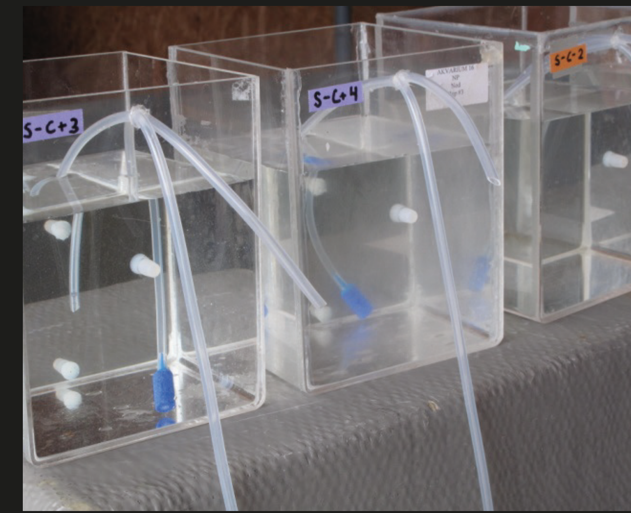
Fig. 3 Experimental setup with 4 litre aquaria, sealed with lids to create headspace and bubbled with synthetic air containing either 380 ppm CO 2 or 960 ppm. Green mesh covers to reach PAR values similar to a depth of ~5m.
