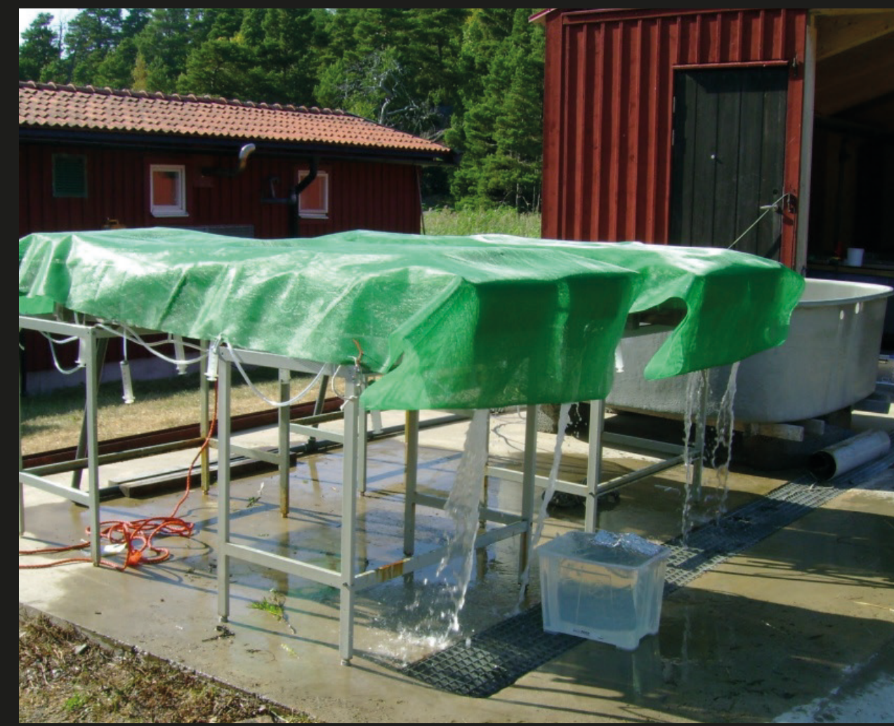
Fig. 3 Experimental setup with 4 litre aquaria, sealed with lids to create headspace and bubbled with synthetic air containing either 380 ppm CO 2 or 960 ppm. Green mesh covers to reach PAR values similar to a depth of ~5m.
