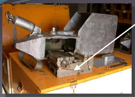
An internal cassette fits into the towing body
