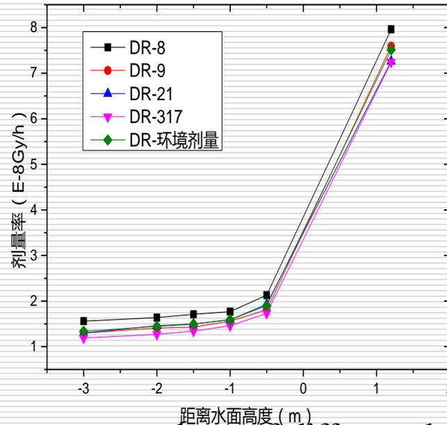
We compared the measurement data of different depths below the surface, the water environmental dose rate increases weaken with depth change, especially in the depth below 1.5m, that shows the shielding effect is stabilized by water.
