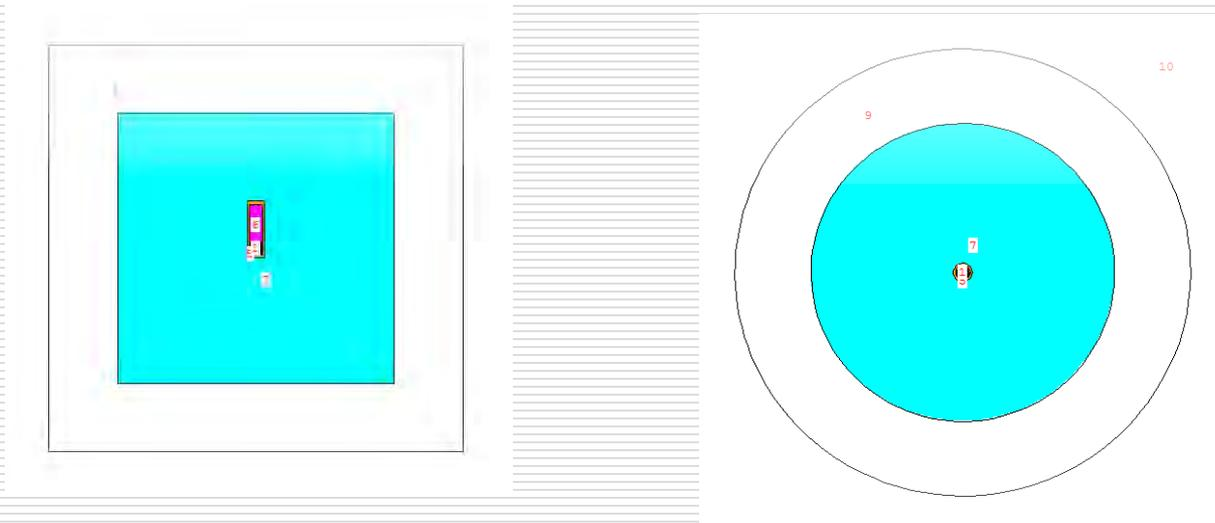
The figure shows the Monte Carlo model we established. By using this model, we can calculate the relationship between different concentrations of  $^{137}\text{Cs}$  activity and dose rate change with a stable effect from  $^{40}\text{K}$  and other natural radionuclides. Then we verified by performing experiment.
