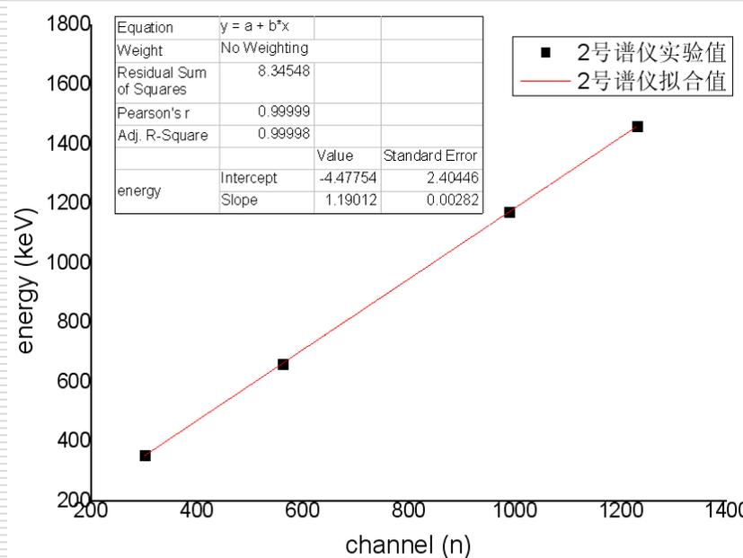
Instrument energy calibration curve fitting formula is:  $E_{\gamma} = 1.19Ch - 4.478$ , correlation coefficient R is 0.999 。
