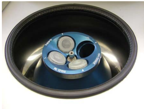
Centrifugation: to separate eggs from heavier particles
