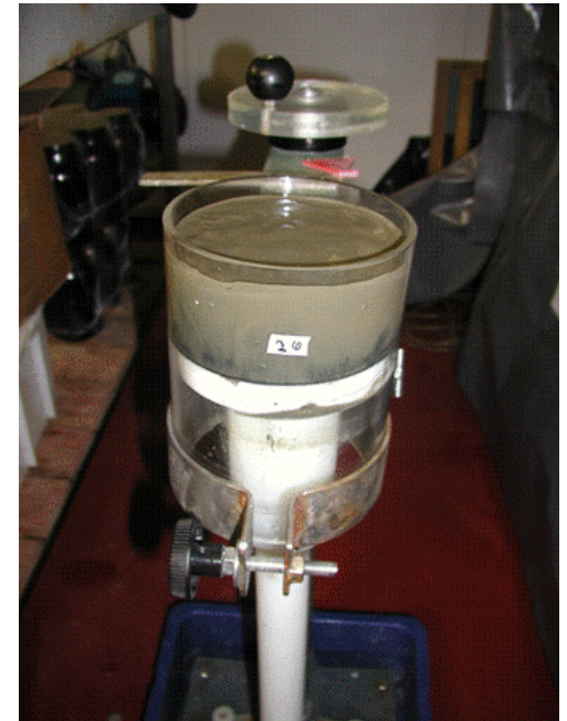
Effects of macrofauna on the depth distribution of cladoceran eggs: cylinders with a movable bottom
