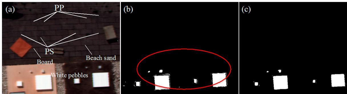
Fig. 10 Results of the photographing experiment (original image of the objects (a), result that the objects were extracted using the references of three bands (b), result that the objects were extracted using the references of all eight bands (c)). Red ellipse in panel (b) denotes misdetection of white pebbles.
