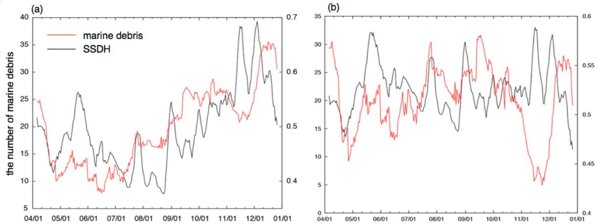
Fig. 4 Comparison of the quantity of beach litter with SSDH (a) and after removing the seasonal variation (b).
