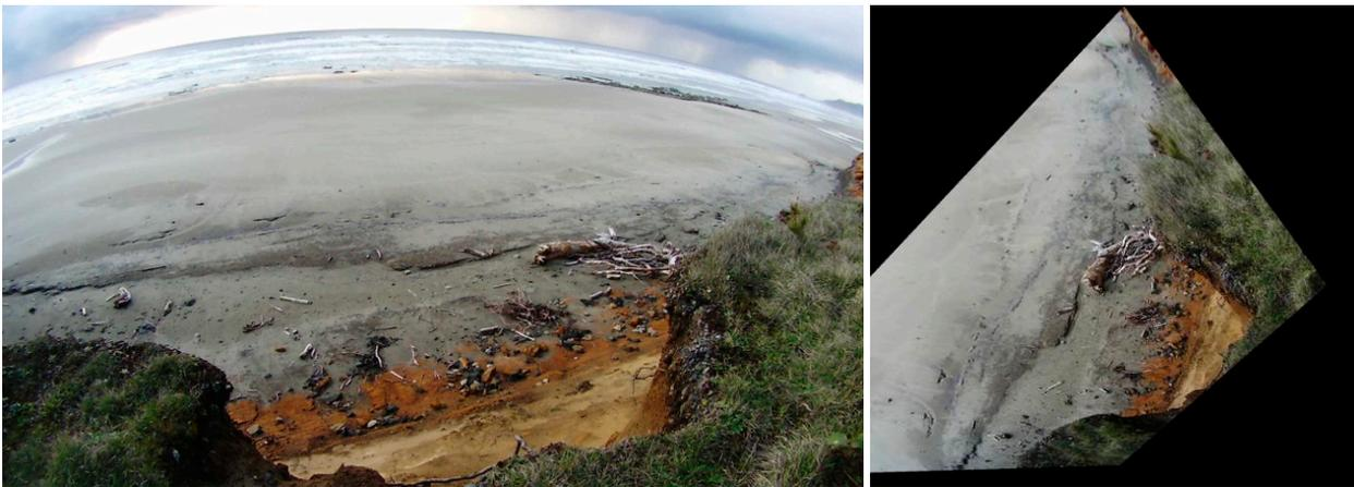
Fig. 2 Original photograph taken by webcam (left) and photograph after applying the projection transformation method (right).
