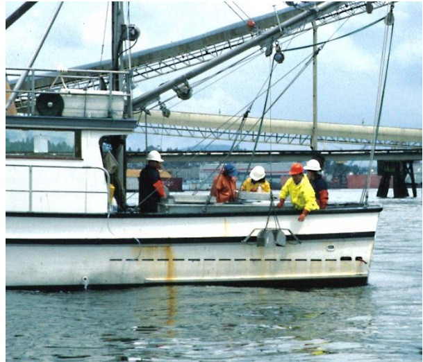
Fig. 1.11 Sediment grab being lowered over the side of the research vessel.
