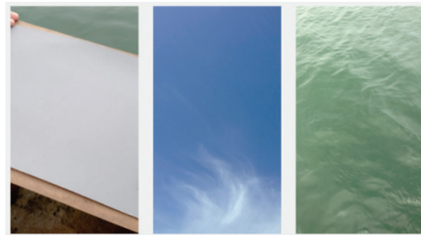
Fig. 1 Example images of the 18% photographer’s grey card (left), the sky (middle), and the water surface (right) collected by a HydroColor user for calculating the remote sensing reflectance ( http://misclab.umeoce.maine.edu/research/HydroColor.php ).
