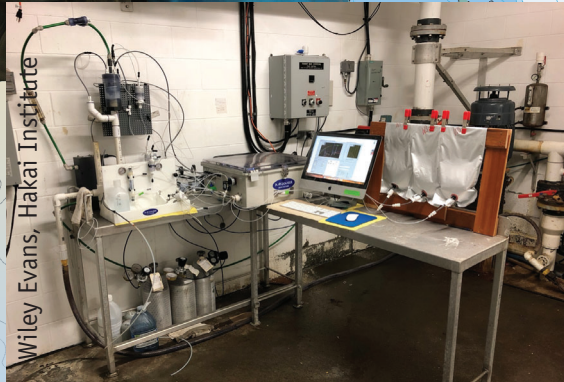
Coastal ocean acidification seawater monitoring using a combined pCO_2 / TCO_2 analyzer at Fanny Bay Oysters in Baynes Sound.
